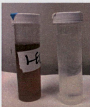
Figure 3. Landfill leachate (left) and SCWO treated effluent (right). Effluent is odorless.
